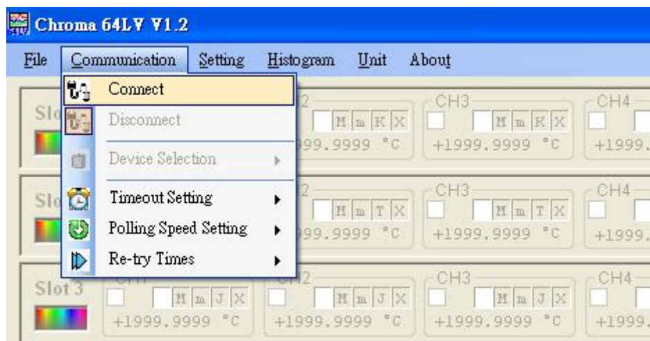
Figure 2-2 Use “Communication” to establish communication
